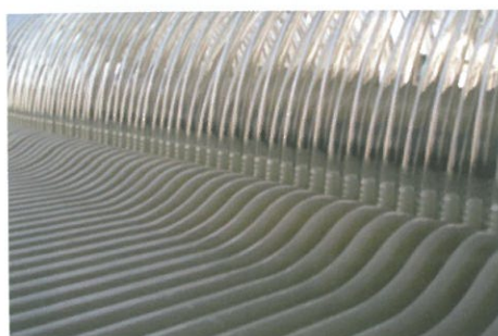
MBR MEMBRANE MODULE PERMEATE MANIFOLD - DETAIL
