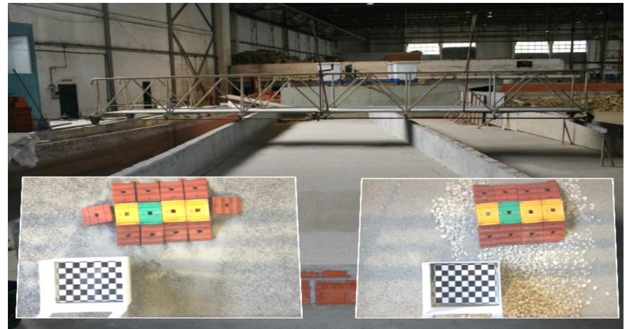
Submerged reef stability: structural sinking and bed erosion
