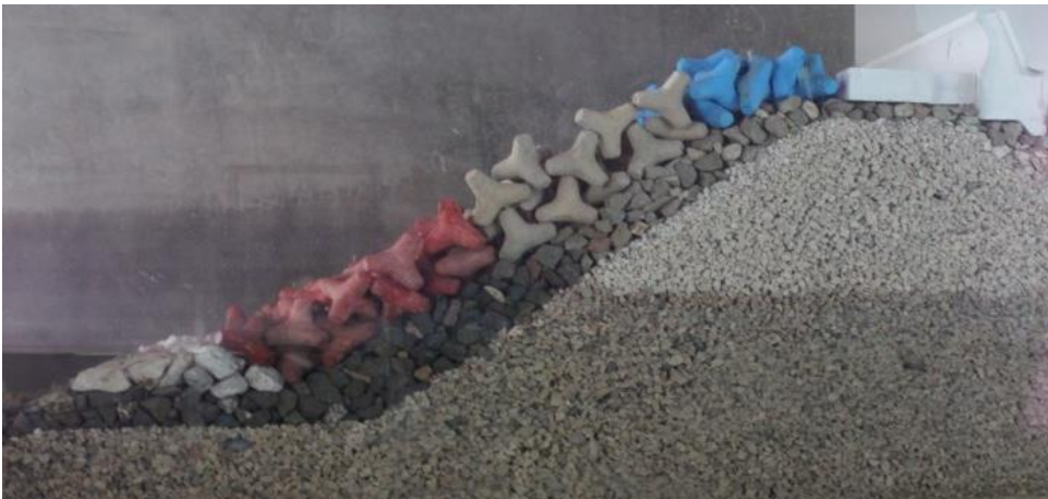
Damage progression analysis using a stereo-photogrammetric survey technique
