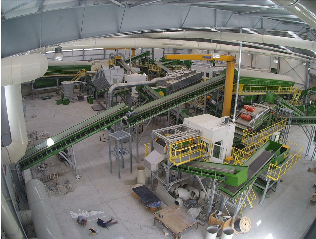
SORTING AND ANAEROBIC DIGESTION OF MSW 150.000 ton/year - MALTA
