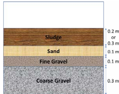
Figure 1. Materials and composition of the drying bed
