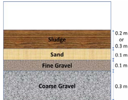
Figure1. Materials and composition of the drying bed
