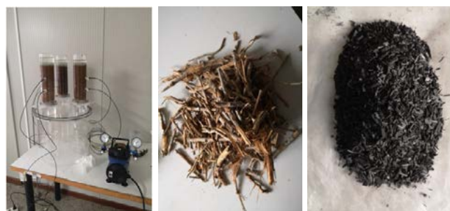
Figure 2. Details of the unsaturated-infiltration columns, woodchips from pruning remains and biochar
