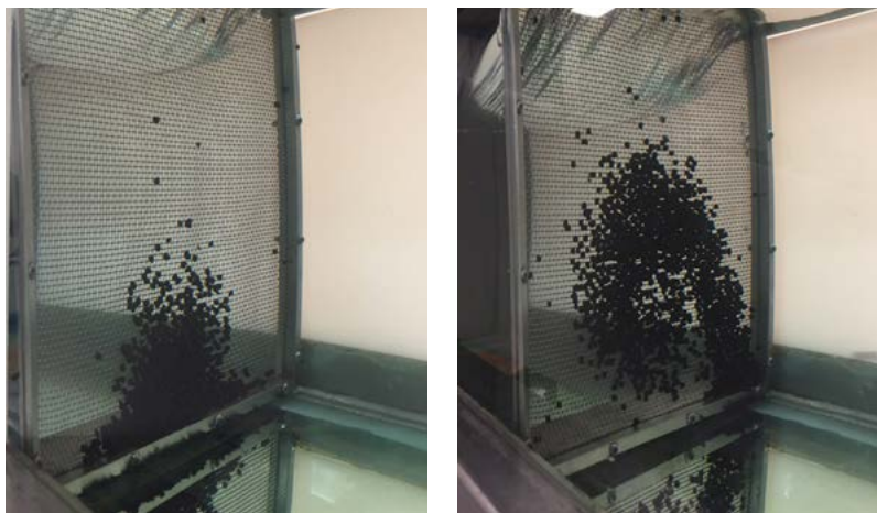
Figure 8. Comparison of particle dispersion in a hydrodynamic channel without blades (left) and with SBTech blades (right).
