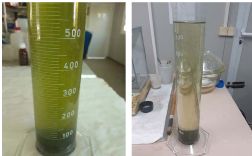
Figure 11. Settling of the reactor content before and after the implantation of the SBTech blades.
