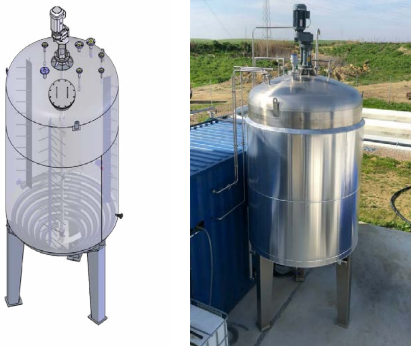
Figure 3. 8 \text{ m}^3 fermentation tank. Scheme (left) and image of the equipment installed in the fermentation unit, outside the maritime container (right).
