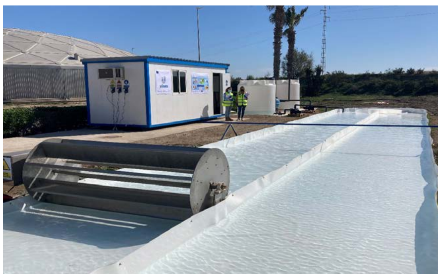
Figure 3. Solar photo-Fenton RPR tertiary treatment plant at demonstrative scale (LIFE ULISES project, grant agreement no. LIFE18 ENV/ES/000165). Scheme of the redox cycle of the solar photo-Fenton process.
