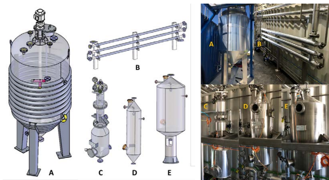
Figure 2. The figure shows the different systems that integrates the pretreatment system. A – Buffer tank; B – Tubular heat exchanger; C – C&F device; D – Flash 1; E – Flash 2.
