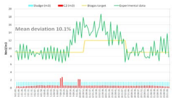
Figure 2. Example of comparison between target biogas production and experimental biogas production in continuous digesters
